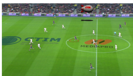
Figure 10: Graphic insertion with camera calibration using tripod geometry and primitive tracking. Extracted from the videos provided as supplementary material ( http://www.ctim.es/demo104/ ).
