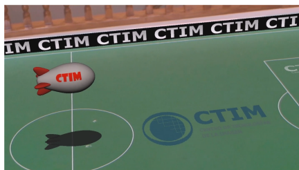
Figure 9: Graphic insertion with camera calibration using tripod geometry and primitive tracking. Extracted from the videos provided as supplementary material ( http://www.ctim.es/demo104/ ).
